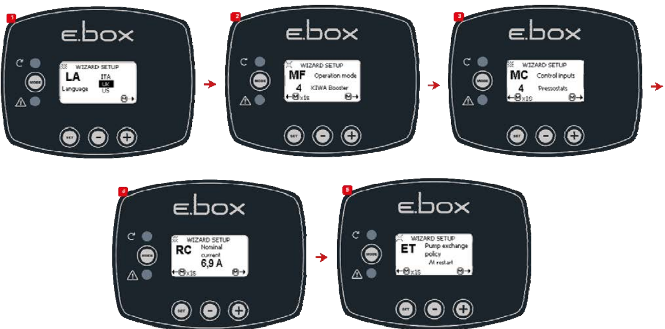
Figure 49: Kiwa configuration with pressure switches
