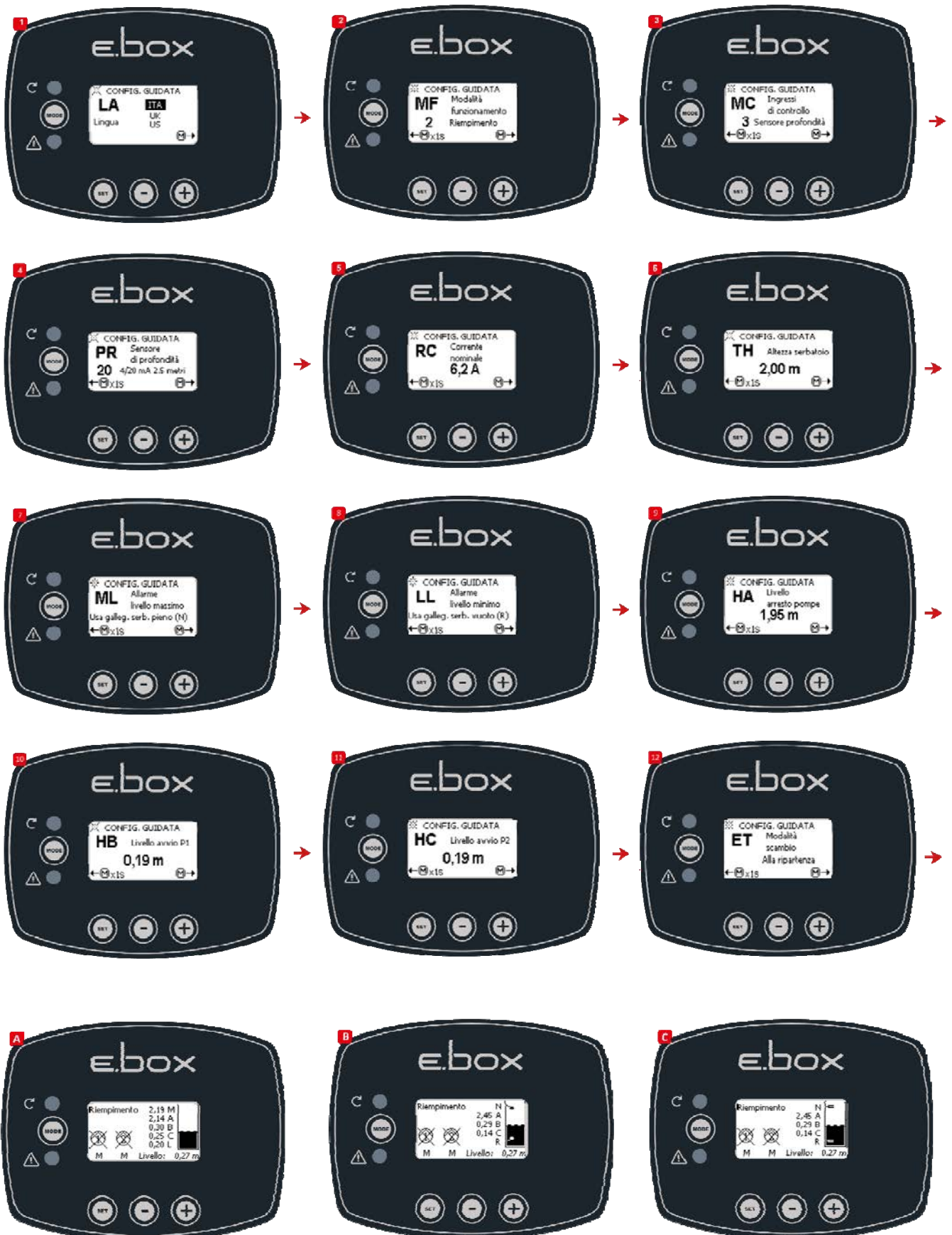
Figure 26: A System status with depth sensor only, B depth sensor and floats, C depth sensor and level probes
