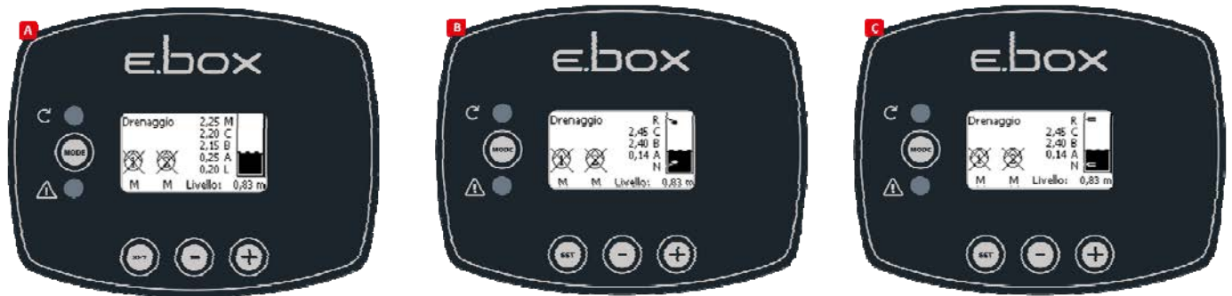
Figure 39: System status in configurations: A with only depth sensor, B: depth sensor and floats, C depth sensor and level probes
